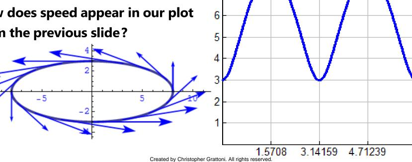
Why do the acceleration vectors point inward? If this particle were a train on an elliptical track, describe how you'd experience these acceleration vectors as a passenger on the train.  $P(t) = (8\cos(t), 3\sin(t))$
